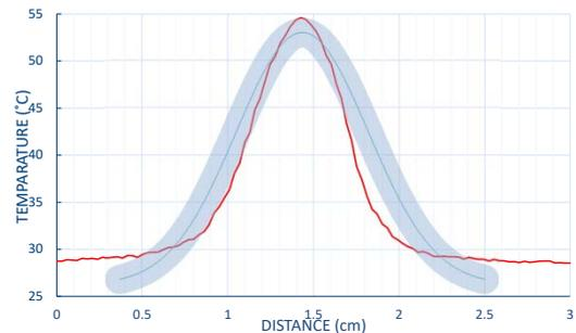
Fig. 4 Correlation between the optical and thermal images (Kapton substrate with 0.054 Watt input power). The red curve represents the output from the IR camera, while the blue curve represents the mean grey-scale value that was extracted from the optical camera. The shaded area indicates the standard deviation of the grey-scale determination.
