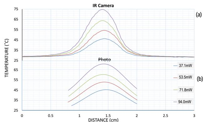
Fig. 5 Comparison of the temperature and grey-scale distribution, as extracted for the thermal (a) and the optical (b) images respectively.
